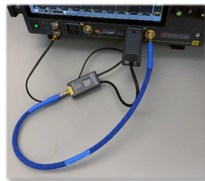
PrecisionProbe characterization of a 1.85 mm cable to 70 GHz using the N2126A calibration module
