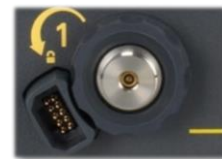
Ruggedized 3.5 mm Male Bulkhead Connector with AutoProbe II Interface
